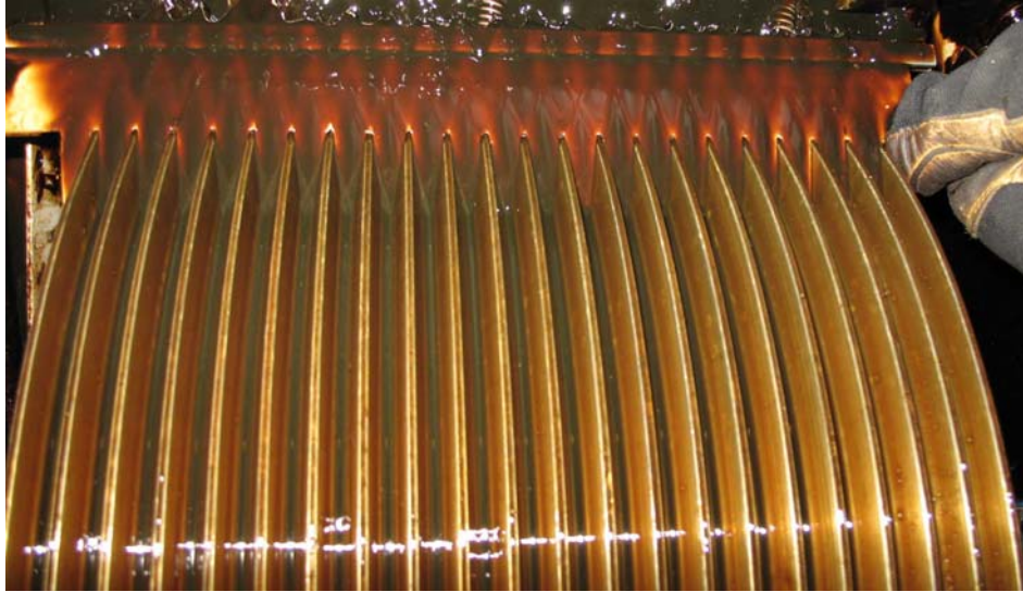
Figure 50. Recovery of diesel with the 30° grooved drum. Note that only a fraction of the groove is occupied with diesel, indicating that a narrower groove would recover significantly more diesel.
