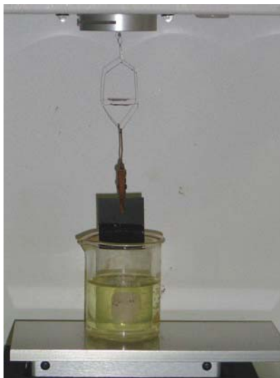
Figure 8. Thermo Cahn Radian 315 measuring oil recovery.
