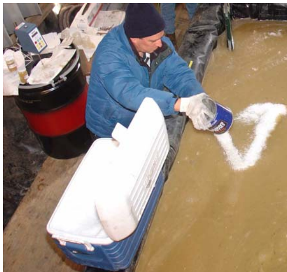
Figure 33. Addition of ice to the oil (HydroCal 300) in the test tank.
