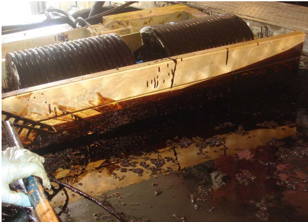
Figure 46. Minimal ice buildup behind (a) Mini Max skimmer and (b) PE 118 skimmer.
