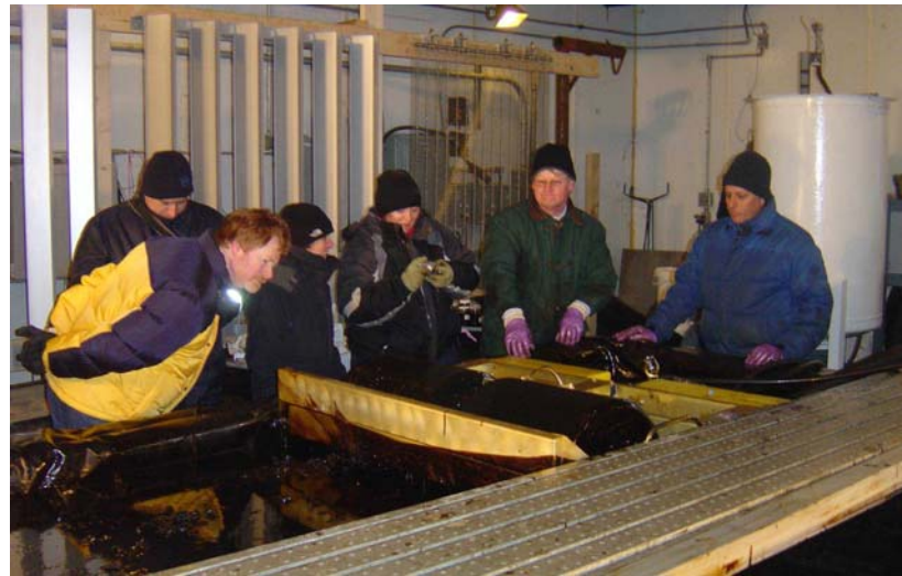
Figure 11. MEF facility at CRREL (a) test tank with Mini Max skimmer; (b) skimmer operation during recovery tests.
