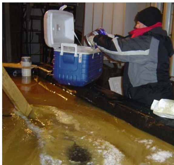
Figure 39. Mixing of ice with HydroCal 300 in circular motion.
