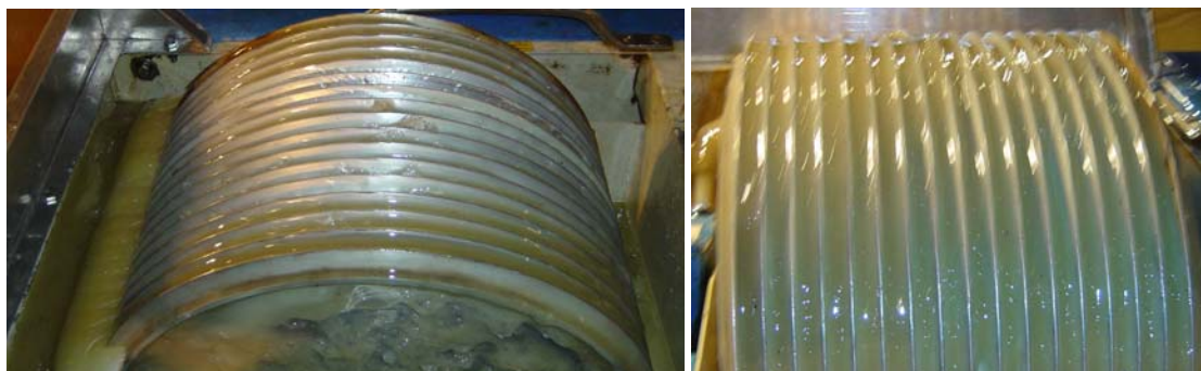
Figure 40. Ice lifted out of the oil/ice mixture along with HydroCal 300.
